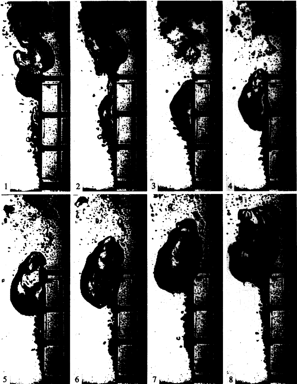
FIG. 6. Discharge of air at v_a = 1 \text{ m s}^{-1} into water from a vertical rectangular nozzle ( H = 10 \text{ mm} , W = 10 \text{ mm} ) stretched with a 600-mesh gauge of stainless steel wire.
